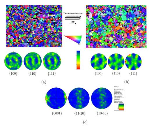
Fig. 2. EBSD mappings of grain orientations in the rolling direction plane; the dark phase corresponds to TiB<sub>2</sub> particles. (a) Cold rolled composite, (b) Hot rolled composite and (c) Crystallographic texture of the TiB<sub>2</sub> particles.
