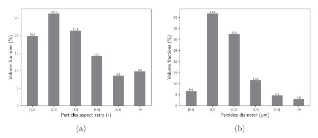
Fig. 4. Results of the SEM image analysis for the hot rolled Fe–TiB<sub>2</sub> composite. (a) Distribution of the particles' aspect ratios in the RD and (b) Distribution of the particles' diameters in the TD.
