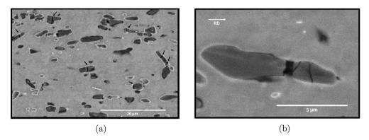
Fig. 5. SEM micrographs of Fe–TiB<sub>2</sub> cold rolled composite. (a) Typical microstructure showing several cracked particles in the cold rolled composite (indicated by arrows) and (b) Example of a cracked particle in the cold rolled composite.
