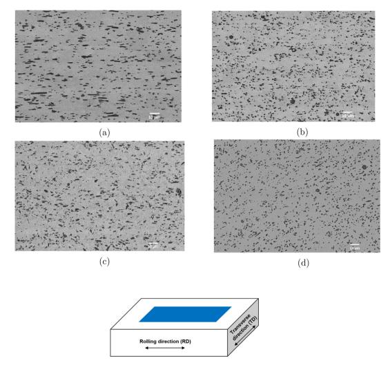
Fig. 1. SEM (image mode: BSE) micrographs of Fe–TiB<sub>2</sub> composite (TiB<sub>2</sub> particles appear with dark contrast). (a) Hot rolled, rolling direction, (b) Hot rolled, transverse direction (c) Cold rolled, rolling direction, (d) Cold rolled, transverse direction.
