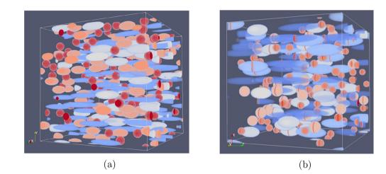
Fig. 6. Microstructure reconstruction of Fe–TiB<sub>2</sub> composite after SEM image analysis (RVE size =  $512^3$  voxels). (a) Hot rolled composite and (b) Cold rolled composite.
