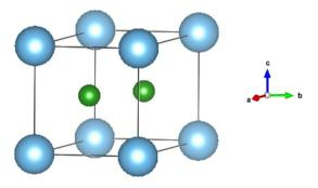
Fig. 3. Hexagonal crystal structure of titanium diboride.
