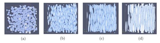
Fig. 7. Randomly generated spheroidal (prolate) particles with a volume fraction of 10%. (a) Aspect ratio of 1, (b) Aspect ratio of 3, (c) Aspect ratio of 6 and (d) Aspect ratio of 9.
