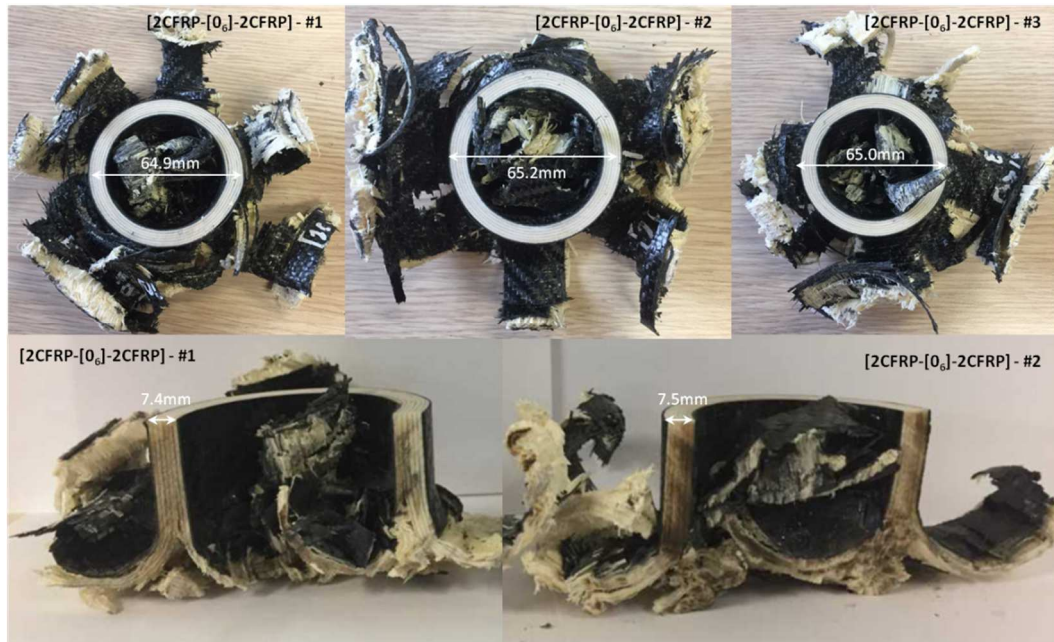
Fig. 8. Failure pattern of tubes [2CFRP-[0 6 ]-2CFRP] and tubes #1 and #2 after cutting.
