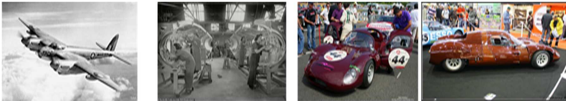
36 Fig. 1. The mosquito and its manufacture in two half fuselages, and the Costin-Nathan with a wooden frame, 1100 37 cm 3 , 410 kg.
