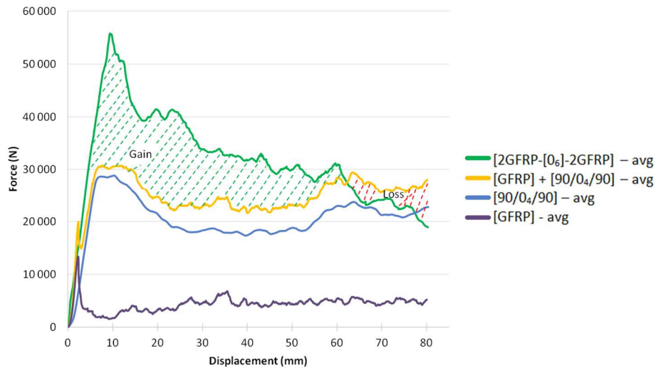
Fig. 24. Static coupling for a sandwich [2GFRP-[0 6 ]-2GFRP]
