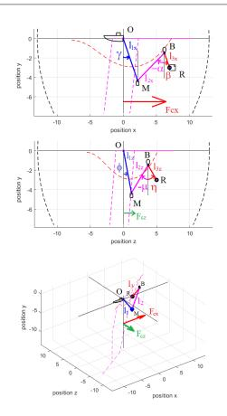
**Figure 13.** Parameters for Sea Exploration with current in 3D case, for (x, y, z) = (5, 2.5, 3). *M*: fixed ballast. *B*: sliding buoys. The blue, magenta, red lines correspond to  $l_1$ ,  $l_2$ ,  $l_3$ . Black dash line: area where the ROV can move due to the umbilical length. Red and green arrows: horizontal currents  $F_{cx}$  and  $F_{cz}$  in direction  $\vec{Ox}$  and  $\vec{Oz}$  with  $F_{cx} = 3F_{cz}$ .
