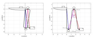
(a) Collision due to umbilical rigidity (b) Absence of collision
