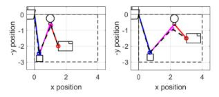
**Figure 22.** Comparison between theoretical umbilical (colored plain lines) and measured umbilical (large dash black lines). Small black dash lines: poolside. Left:  $E_B = 0.107$ m. Right:  $E_b = 0.327$ m, largest discrepancy of the experimentation.
