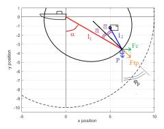
**Figure 4.** Parameters for Surface Exploration with horizontal current. *M*: sliding ballast. Black dash line: area where the ROV can move due to the umbilical length. Solid black line: ellipse of centers *O* and *R* and radius  $\frac{L}{2}$  and  $\sqrt{\left(\frac{L}{2}\right)^2 - \frac{x^2+y^2}{4}}$ .
