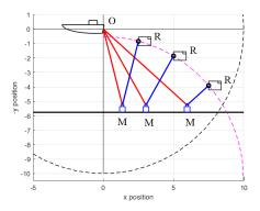
**Figure 3.** Limit depth  $y_{\text{lim}}$  which guarantee the ballast is not in contact with the seafloor for Surface Exploration. *M*: sliding ballast. The dash magenta line:  $y_{\text{lim}}$ . Large black line: seafloor  $y_{\text{floor}}$ . Red line:  $l_1$ . Blue line:  $l_2$ .
