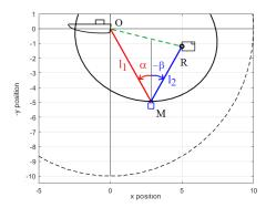
**Figure 2.** Parameters for Surface Exploration. M: sliding ballast. Black dash line: area where the ROV can move with its umbilical of length L. Black line: ellipse of centers O and R. Green dash line: longest diameter of the ellipse.
