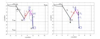
**Figure 16.** Parameters of diving exploration strategy. *M*: fixed ballast. *B*1: sliding buoys. *B*2: fixed buoy.  $P = F_{b1}$  and  $F_{b2} = 63 P$ . Black dash lines: exploration area where the ROV can move due to the constraint taken for umbilical shape.
