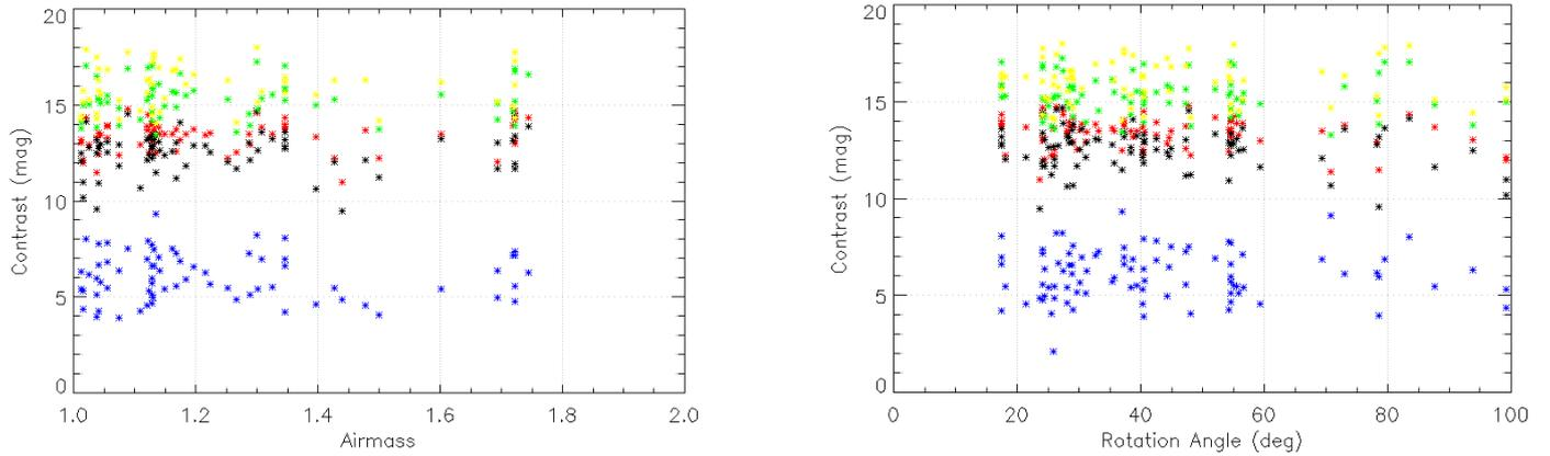
**Fig. B.2.**  $5\sigma$  IRDIS processed contrasts at various separations computed using TLOCI estimated as function of the observing conditions (airmass and rotation angle) in irdifs mode. Blue is for 100 mas separation, black for 500 mas separation, red for 1000 mas separation, green for 2000 mas separation, and yellow for 4000 mas separations.
