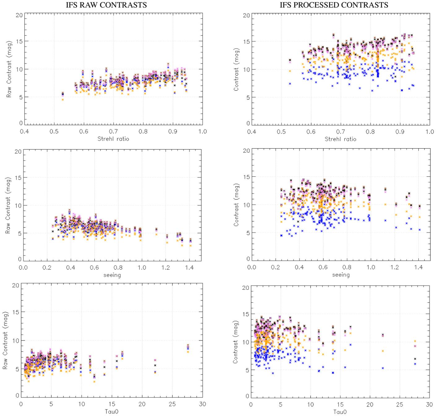
**Fig. B.4.** IFS raw (*left*) and processed (*right*) contrasts in *YJ* bands at various separations computed using PCA ASDI estimated as function of the observing conditions in irdifs mode. Blue is for 100 mas separation, orange for 200 mas separation and pink for 400 mas separations, black for 500 mas separation, brown for 700 mas separation.
