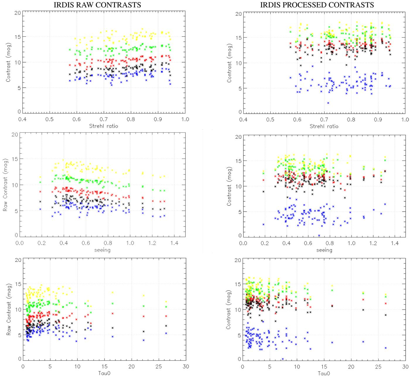
**Fig. B.1.** IRDIS raw (*left*) and processed (*right*) contrasts in H2 band at various separations, computed using TLOCI estimated as function of the observing conditions in irdifs mode. Blue is for 100 mas separation, black for 500 mas separation, red for 1000 mas separation, green for 2000 mas separation, and yellow for 4000 mas separations. The seeing is expressed in arcseconds and the  $\tau_0$  in milliseconds.
