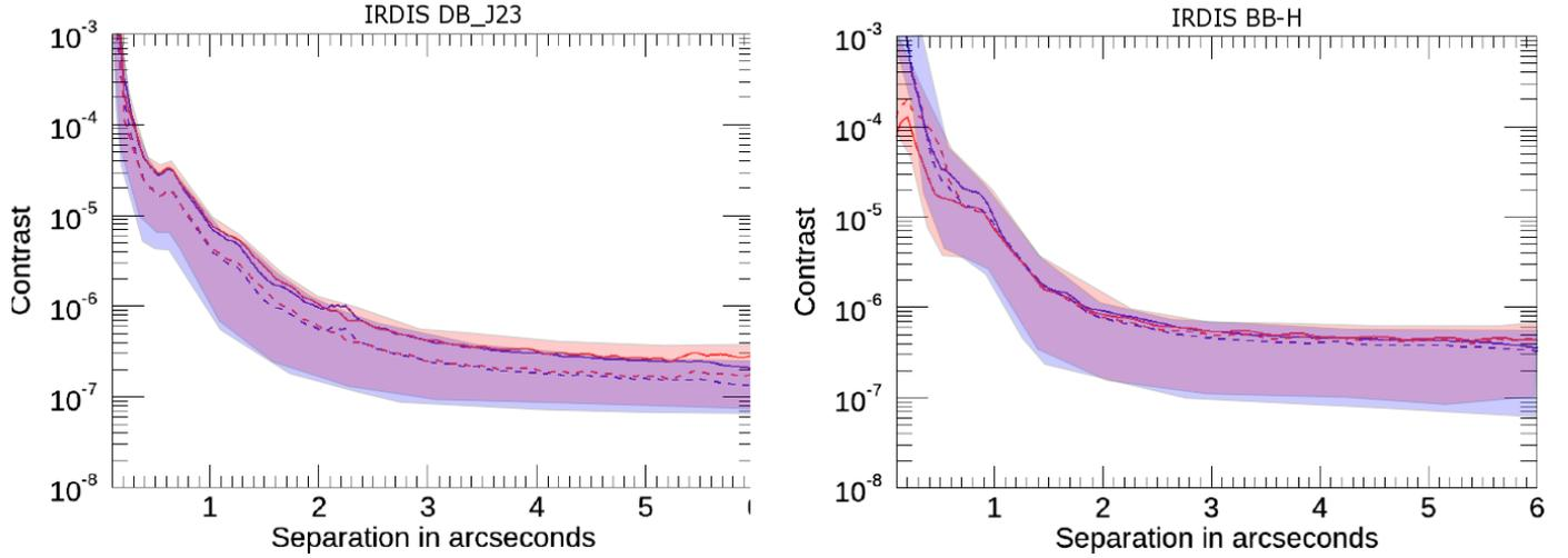
**Fig. 5.** Contrast curves at  $5\sigma$  obtained for a small subsample of targets dedicated to follow up for IRDIS mode observations. The solid line gives the median value of the contrast. The dashed line gives the mean value of the contrast. Red indicates IRDIS data reduced in PCA ADI; blue indicates IRDIS data reduced in TLOCI ADI; and green indicates IFS with a PCA ASDI reduction.
