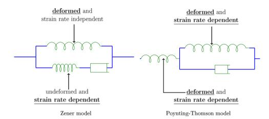
Fig. 2. Comparison of the state of each elements in rheological schemes of Zener and Poynting-Thomson models after a static deformation.
