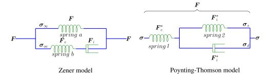
Fig. 1. Notations used in the Zener model and the Poynting-Thomson model for large strain formulation.
