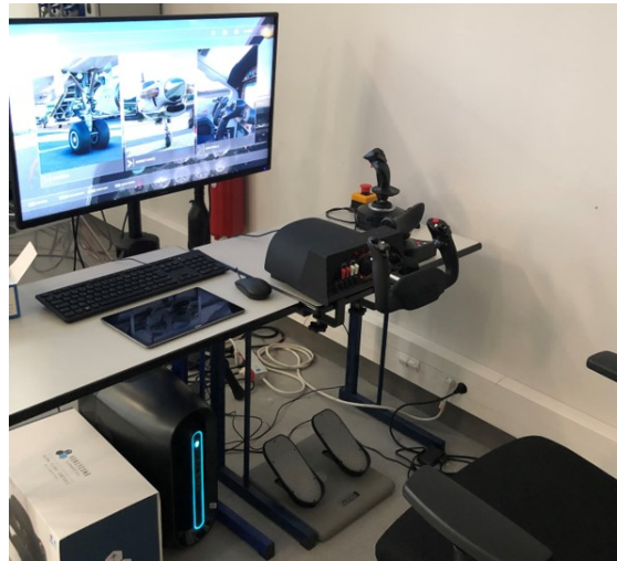
Fig. 2. The experimental setup: FlightSimulator2020 displayed on a computer screen, yoke, pedals, joystick and the tablet.
