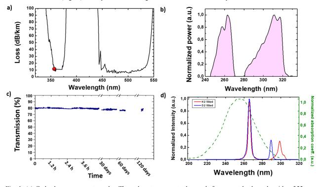
Fig. 1: (a) Cutback measurement results. The red spot represents the result from a cut back made with a 355 nm laser. (b) Normalized transmissions in the UV measured with a plasma lamp. (c) Fiber lifetime measurement under UV radiation over 120 days. (d) Raman generation plots in a 25 cm  $D_2$ -filled fiber (blue curve) and in a 7 cm  $H_2$ -filled fiber (red curve). The green curve represents the normalized absorption coefficient of the ozone in the Hartley band.
