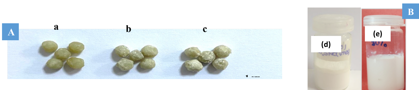
Figure 1. (A): Images of: uncoated DAP (a), DAP coated with PBMA 8% SNC (b) and DAP coated with P(BMA-co-PFA) 8 wt % SNC (c). (B): Visual aspect of: PBMA (d) and P(BMA-co-PFA) (e) dispersions after emulsion (co)polymerization in the presence of 8 wt % SNC.
