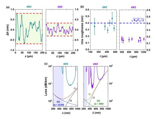
Fig. 3. (a) Typical core surface roughness profiles ( $\Delta h$ : roughness height variation) and (b) measured rms roughness. (c) Typical loss spectra for fibers in G#1 and G#2; Confinement loss (CL), surface scattering loss (SSL) and total loss (TL) trends.
