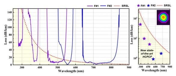
Fig. 2. F#1 and F#2 measured loss together with the silica Rayleigh scattering limit (SRSL) trend and a typical output near field profile.
