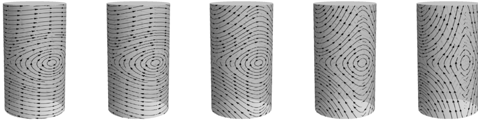
FIGURE 6. Phase portrait of the Eringen's nonlocal elastica for \beta = 1 , l = 0 , l = 0.2 , l = 0.5 , l = 0.7 and l = 0.9
