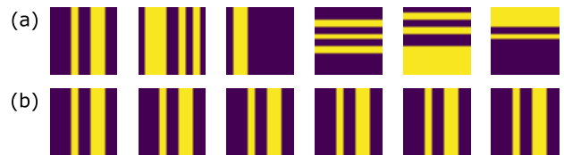
FIG. 14. Visible configurations obtained with Alternating Gibbs Sampling and Metropolis-Hastings algorithm in the hidden space, L = 10 . 25 Gibbs steps between each frame. (a) With L_1 regularization. (b) Without L_1 regularization.
