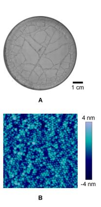
FIG. 1. (A) Crack patterns of a dried colloidal layer. (B) Topographical AFM image of the top surface of the layer (scan size  $500 \times 500 \text{ nm}^2$ ). The sample pictured here was dried at RH = 50%.
