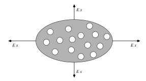
FIG. 4. Representative Elementary Volume (REV) corresponding to a homogeneous matrix with spherical pores submitted to displacement Ex along its boundary, with E the strain tensor and x the position vector.
