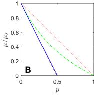
FIG. 5. Predictions of the different schemes for  $\nu_s = 0.16$  (pure silica): rule of mixtures (red dotted line), Eshelby's approximation (brown dash-dot line), Mori-Tanaka scheme (green dashed line) and self-consistent scheme (blue solid line).
