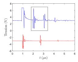
FIG. 9. Time evolution of the signal received at the transducer for compression waves (blue) and shear waves (bottom). The material probed here is a sample dried at RH=50% and the specimen thickness is  $2.07\pm0.03$  mm. For the sake of clarity, the signals are shifted by 3 V and -3 V respectively. The black box delimits the signal represented on Fig. 10.
