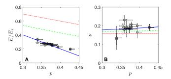
FIG. 7. Normalized Young modulus (E) and Poisson's ratio  $(\nu)$  as a function of porosity (p). The experimental values for E were normalized by the spec value of bulk fused silica glass  $(E_s)$ . Lines correspond to theoretical schemes: rule of mixtures (red dotted line), Mori-Tanaka scheme (green dashed line) and self-consistent scheme (blue solid line).
