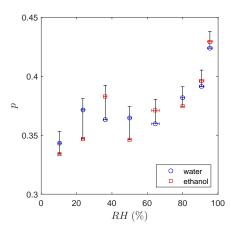
FIG. 2. Porosity (p) as a function of relative humidity (RH), measured by hydrostatic weighing in water (blue circles) and in ethanol (red squares). In the rest of the article, p is taken as the average of these two values. The vertical error bars account for the possible presence of water trapped in the dry samples (Tab. I). The horizontal error bars represent the standard deviation on RH during the drying experiments.
