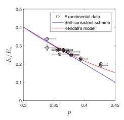
FIG. 8. Normalized Young's modulus as a function of porosity. The numeric values used in Kendall's expression (eqn (22)) were  $E_s = 72.7$  GPa, a = 16.2 nm (measured values) and W = 5 J/m<sup>2</sup> (fitted value for A = 10.3, as used in [12, 13, 15]).
