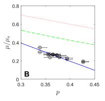
FIG. 6. Normalized bulk modulus  $(k/k_s)$  and shear modulus  $(\mu/\mu_s)$  as a function of porosity (p). Normalization procedure uses bulk fused silica glass parameters (spec values from Tab. III). Lines correspond to theoretical schemes: rule of mixtures (red dotted line), Mori-Tanaka scheme (green dashed line) and self-consistent scheme (blue solid line).
