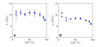
FIG. 3. Bulk modulus (k) and shear modulus  $(\mu)$  as a function of relative humidity (RH). Error bars correspond to standard deviation. For each drying rate, the measurements were repeated on two morsels.
