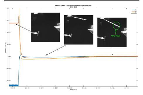
Fig. 9 Time series of magnetic field components during the magnetometer boom deployment on 25/10/2018. Also, pictures from the MCAM are shown for visual checking
