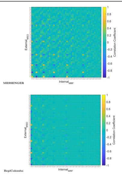
Fig. 26 Correlations between internal Gauss and external coefficients due to the MESSENGER orbit (top) and due to the BepiColombo orbit (bottom). In this figure, the external Gauss coefficients are not capitalized
