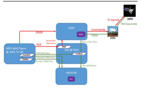
Fig. 7 Simplified schematic overview of the complete process concerning commanding (red) & data retrieval and pipelining (green). Details and acronyms are described in the main text.
