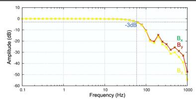
**Fig. 6** Calculated frequency response for the OB sensor at 76 °C for  $B_x$  (green),  $B_y$  (red) and  $B_z$  (yellow).
