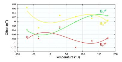
Fig. 5 Temperature dependence of the IB sensor offsets.
