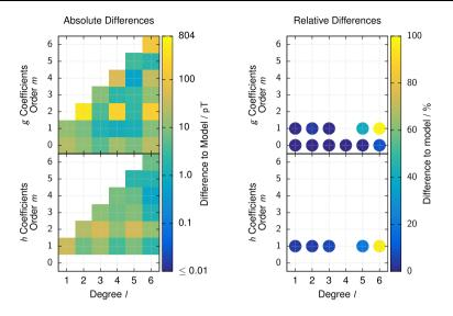
**Fig. 23** Resulting absolute (left) and relative (right) differences of Gauss coefficients with an offset of 1 nT and a sensor rotation around its *x*-axis of 0" — Small offset errors, no sensor rotation
