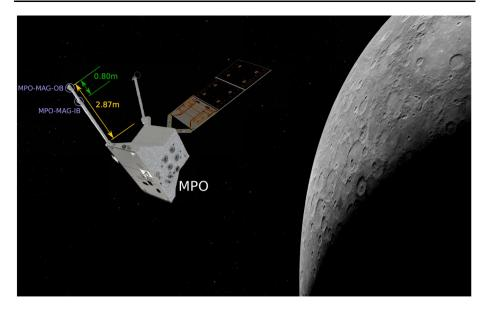
Fig. 2 MPO-MAG locations on the MPO spacecraft at Mercury (artist impression). Image credit: Spacecraft: ESA/ATG medialab; Mercury: NASA/Johns Hopkins University Applied Physics Laboratory/Carnegie Institution of Washington.
