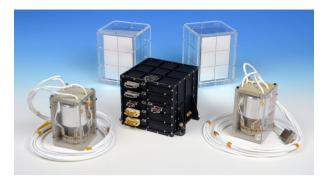
The planetary orbiter (MPO) from BepiColombo will be injected into an initially  $480 \times 1500$  km polar orbit around the planet and carries two 3D fluxgate magnetometers mounted on a boom. These magnetic field measurement will allow us to determine the main field, provide measurements about the magnetospheric structure and its dynamics and further constrain the interior structure as well as the dynamo process that generates the internal magnetic field.
