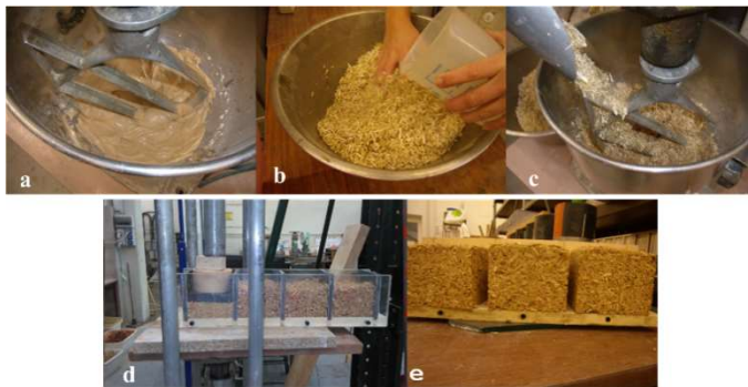
143 144 Fig. 4. Production process: a) Binder mixing (paste); b) Hemp mixing by hand; c) Addition of the moist hemp to 145 the paste and mixing; d) Compaction; e) Designed specimens.
