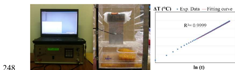
249 Fig. 7. Measurement of thermal conductivity at dry state – left: CT meter and dry chamber, right: experimental 250 thermogram.
