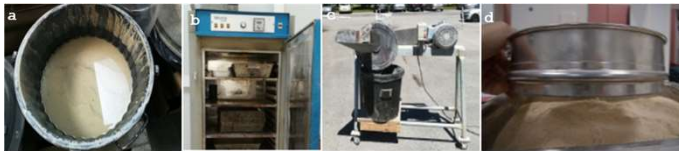
111 Fig. 1. Preparation of clay binder: a) decanting; b) Drying; c) Milling; d) Sieving with a square mesh of 2 mm.
