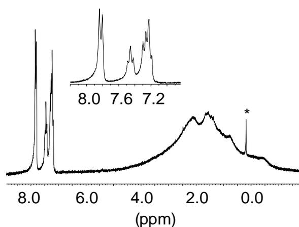
Figure 1.  $^1\text{H}$  NMR spectrum of compound  $(\text{C}_5\text{Pr}_4\text{H})\text{WCl}_4$ . The starred peak is due to a minor diamagnetic contaminant (probably silicone grease)
