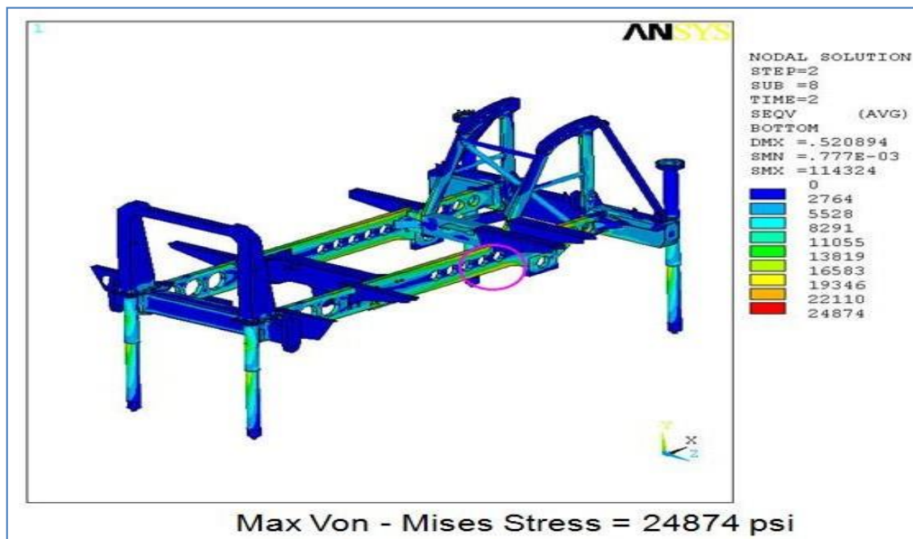
Fig.1.8: Von Mises stress Plot for PV235 Mainframe
