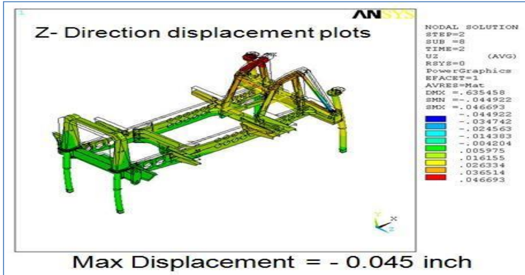
Fig.1.7: Z direction displacement the PV235 Mainframe
