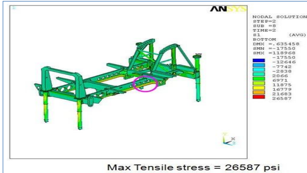
Fig 1.9: First Principal Stress Plot for PV235 Mainframe
