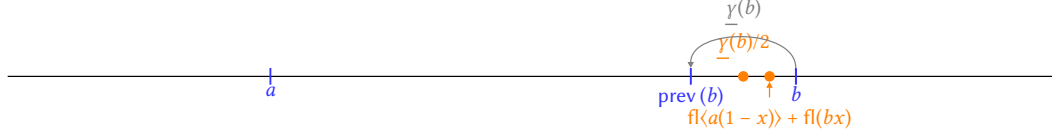
Fig. 7: Conditions for \text{fl}\langle a(1-x) \rangle + \text{fl}\langle bx \rangle to round to b .
