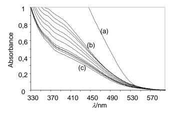
Figure 5. UV-visible study of the interaction between Cp\*Fe(dppe)H and HFIP (5 equiv) in CH<sub>2</sub>Cl<sub>2</sub>. [Fe] = 0.02 M. (a) Before the HFIP addition. (b) T = 270 K. (c) T = 200 K. The other intermediate spectra correspond to 265 - 225 K (5 K step).
