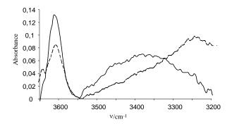
**Figure 2**. IR spectra in the  $v(R_FO-H)$  stretching region showing the interaction between Cp\*Fe(dppe)H and MFE or TFE in CH<sub>2</sub>Cl<sub>2</sub>. Solid line: [Fe] = 0.15 M; [MFE] = 0.015 M. Dashed line: [Fe] = 0.13 M; [TFE] = 0.01 M.
