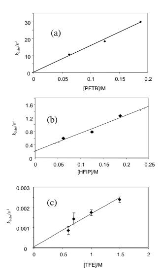
**Figure 7.** Pseudo-1<sup>st</sup> order rate constants for the first step of the proton transfer from HA to  $Cp*Fe(dppe)H[k_{3obs}; HA = PFTB (a), HFIP (b), TFE (c)].$
