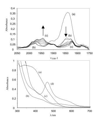
Figure 1. Spectral changes (IR, above; UV-visible, below) observed for the protonation of Cp\*Fe(dppe)H by HBF<sub>4</sub> in CH<sub>2</sub>Cl<sub>2</sub>. (a) Before addition of HBF<sub>4</sub> (T = 200K); (b) after addition of HBF<sub>4</sub> (T = 200K); (c) T = 290 K (after a few minutes); (d) T = 290, after several hours. [Fe] = 0.03 M (IR); 0.01 M (UV-visible); HBF<sub>4</sub>/Fe = 1.
