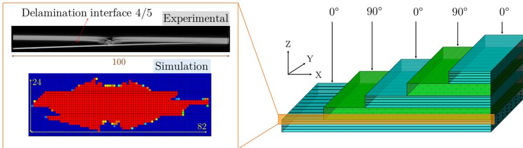
Figure 21: Delamination of the 4<sup>th</sup> interface for the 5P 0-90 at 4 m/s
