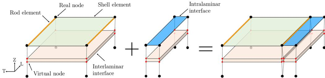
Figure 2: Modelling of the intralaminar interface interspersed between the UD elements
