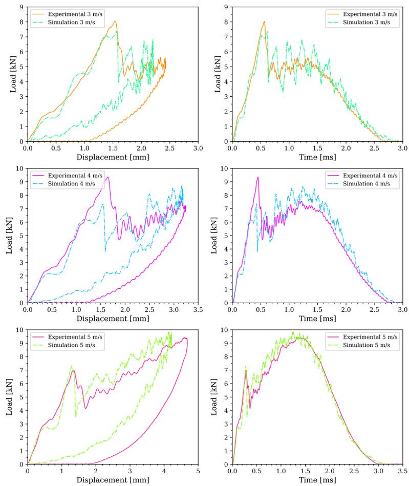
Figure 24: Load-displacement and load-time curves of experimental tests and numerical simulations for 13P 0-90
