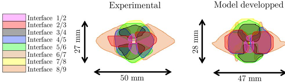
Figure 17: Comparison between experimental and numerical damage
