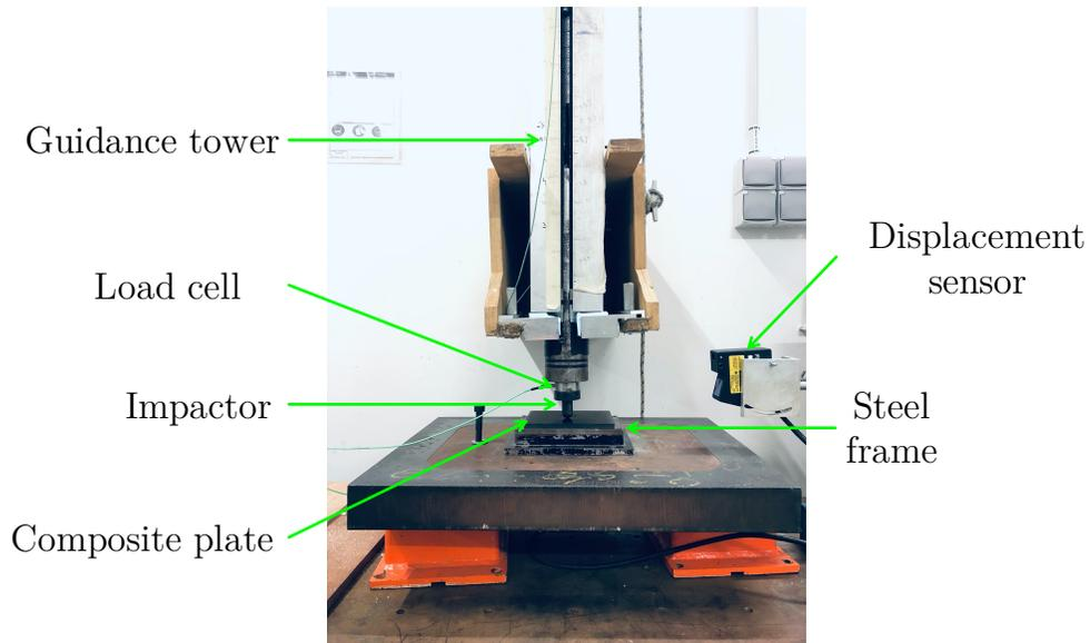
Figure 12: Experimental conditions of the impact tests
