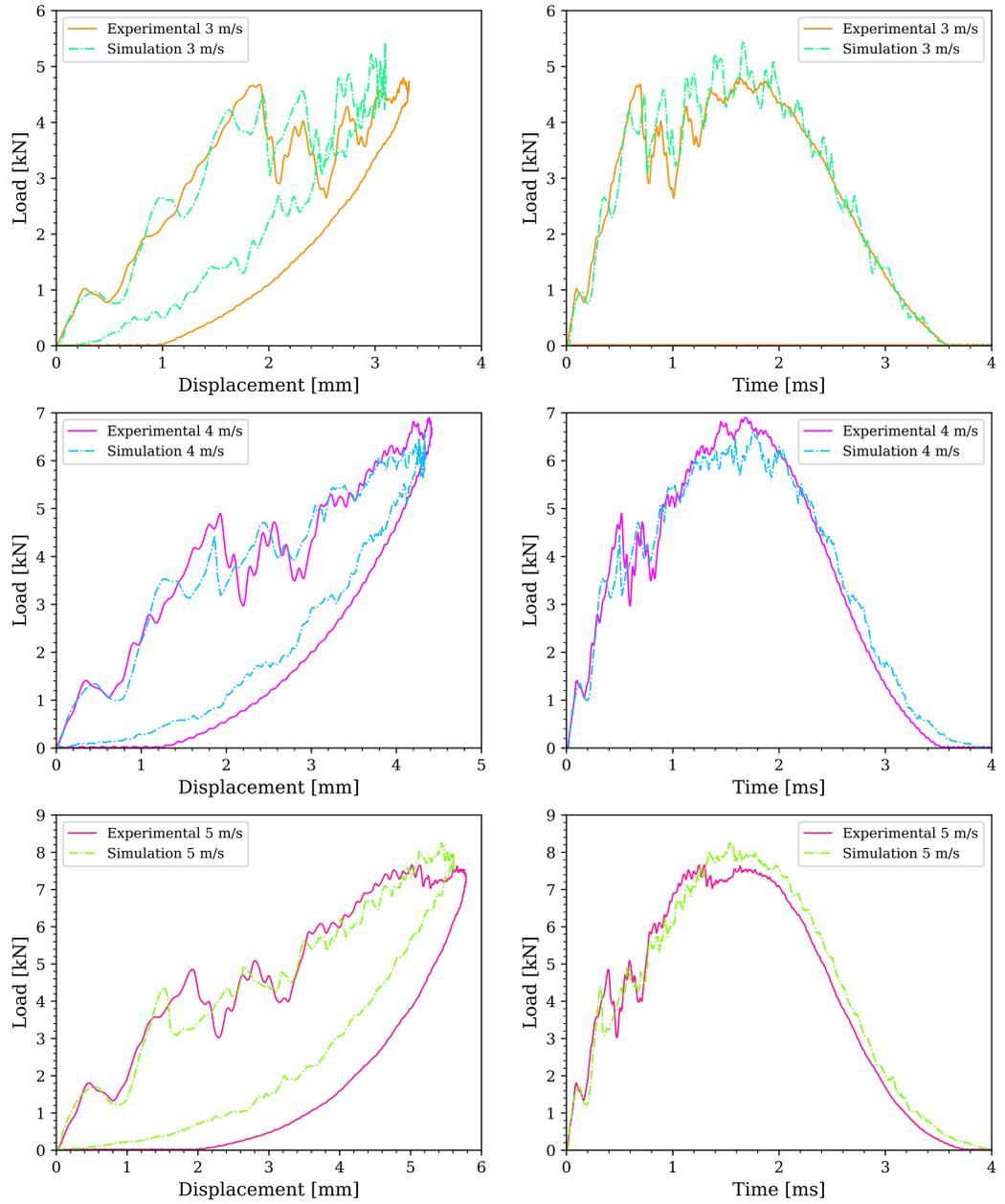
Figure 22: Load-displacement and load-time curves of experimental tests and numerical simulations for “9P 0-90” at 3 m/s, 4 m/s and 5 m/s.
