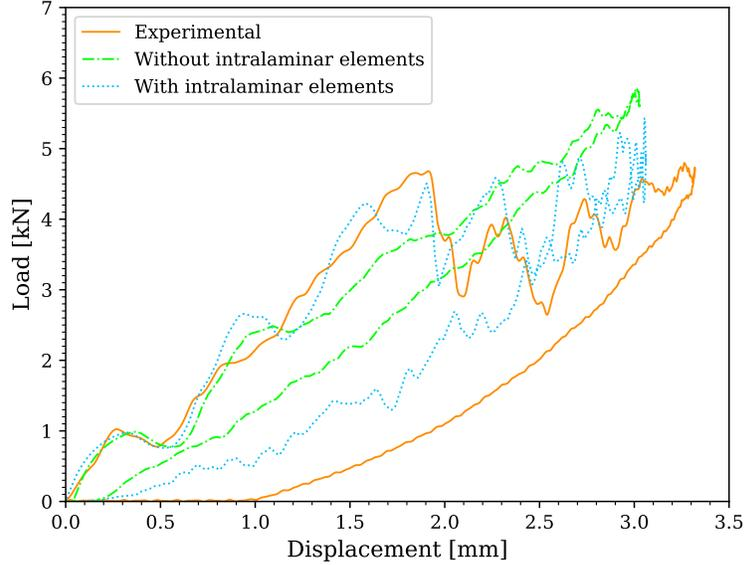
Figure 13: Load-displacement curves for the experimental test and the models with/out intralaminar elements (9P 0-90 at 3 m/s)
