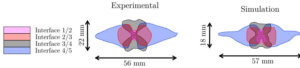
Figure 19: Cartography of the experimental and numerical delaminations for 5P 0-90 at 3m/s
