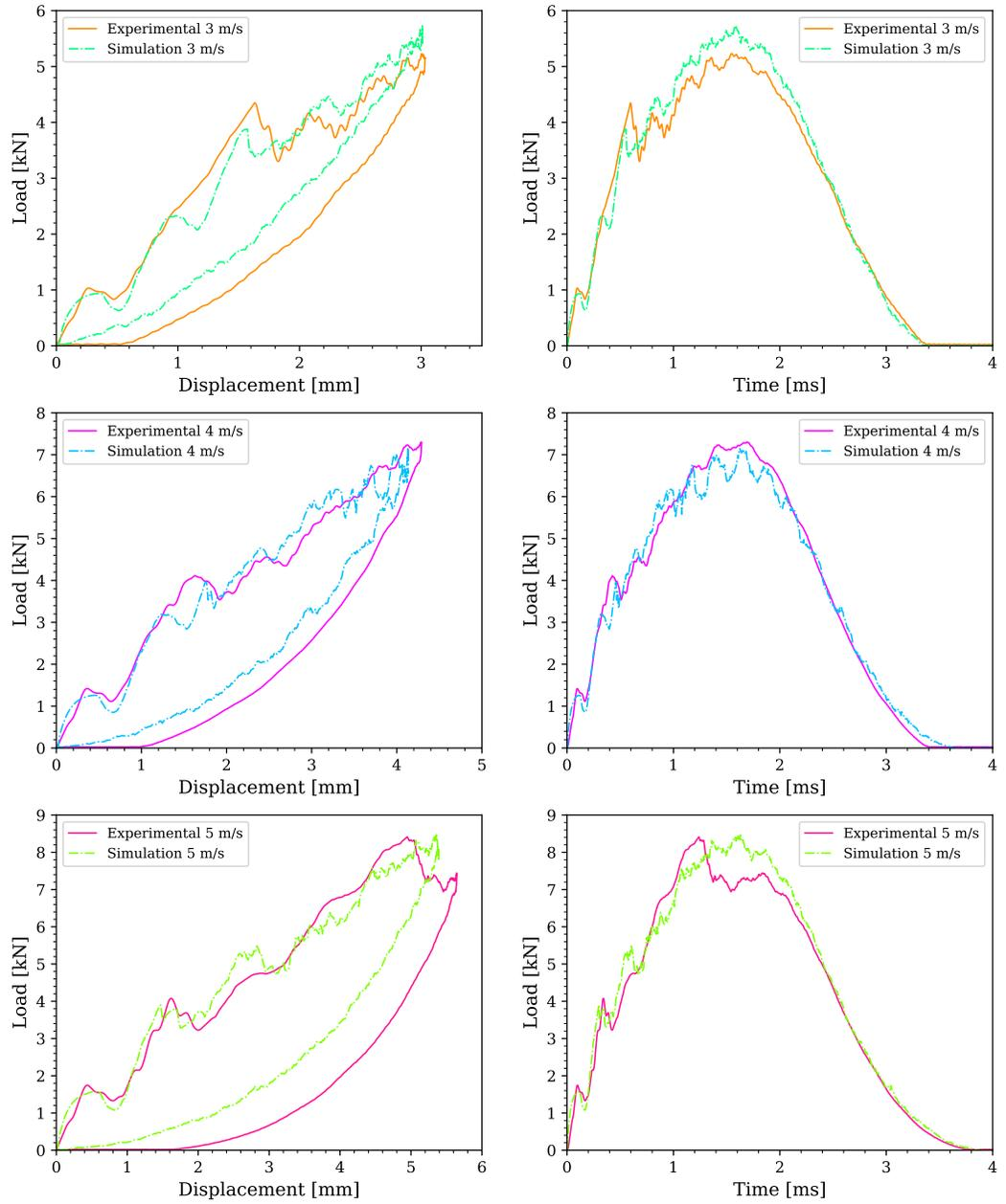
Figure 26: Load-displacement and load-time curves of experimental tests and numerical simulations for 9P QI
