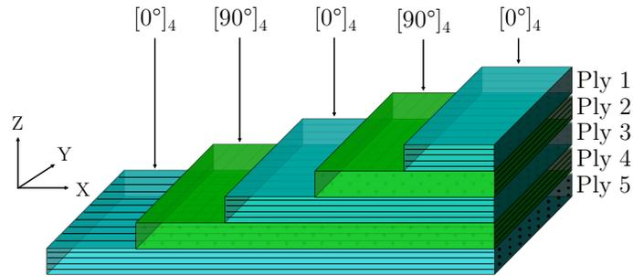
Figure 9: Stacking sequence used for 5P 0-90
