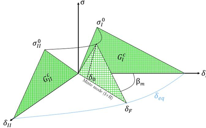
Figure 4: Bilinear cohesive law for the intralaminar interface damage
