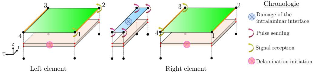
Figure 5: Connexion between intralaminar and interlaminar interfaces
