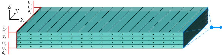
Figure 7: Tensile specimen constituted by four  $90^\circ$  layers
