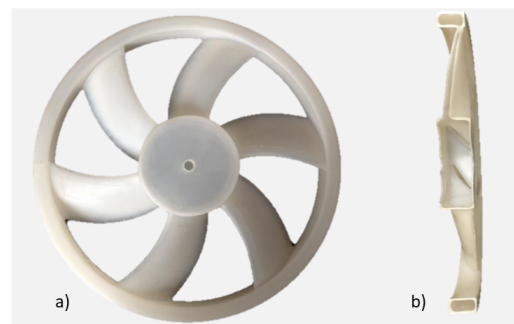
Figure 1. Hollow fan obtained with rotational molding process, (a) the whole fan and (b) the fan cut in two parts [25].
