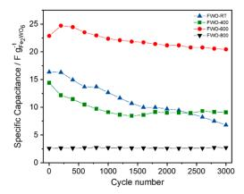
**Figure 4.** Cycling stability up to 3000 cycles at 20 mV s<sup>-1</sup> in 5M LiNO<sub>3</sub> for the selected Fe<sub>2</sub>WO<sub>6</sub> samples.
