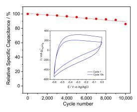
**Figure 5.** Long term cycling stability for FWO-600 sample at 20 mV s<sup>-1</sup> in 5M LiNO<sub>3</sub>. Inset: cyclic voltammograms at cycle 1 and at cycle 10,000.
