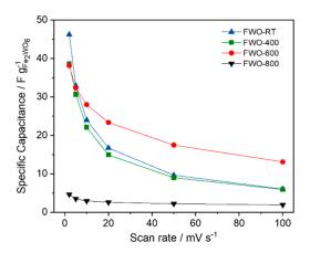
**Figure 3.** Evolution of the specific capacitance in F  $g^{-1}$  vs. scan rate in 5M LiNO<sub>3</sub> for the selected Fe<sub>2</sub>WO<sub>6</sub> samples.
