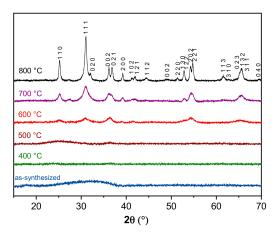
**Figure 1.** Evolution of the XRD patterns of Fe<sub>2</sub>WO<sub>6</sub> synthesized by polyol method from 30  $^{\circ}$ C up to 800  $^{\circ}$ C.
