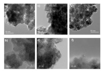
**Figure 6.** TEM images of raw FWO-600 particles (**a**,**b**), after 10,000 cycles (**c**,**d**) and from the blank electrode soaked in the electrolyte (**e**,**f**). Scale bar for figures a, c and e is 50 nm while it is 10 nm for figures (**b**,**d**,**f**).
