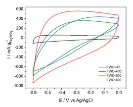
**Figure 2.** Cyclic voltammograms of the samples FWO-RT, FWO-400, FWO-600 and FWO-800 at  $20 \text{ mV s}^{-1}$  in 5M LiNO<sub>3</sub> from 0 to -0.6 V vs. Ag/AgCl.
