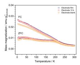
**Figure 8.** T-dependent FC (field-cooled) and ZFC (zero-field-cooled) mass magnetizations for non-cycled "Electrode film", cycled electrode "Electrode 10,000", and non-cycled but soaked in electrolyte "Electrode blank".
