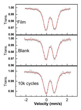
**Figure 7.** Room temperature Mössbauer spectra for non-cycled FWO-600 electrode ("Film"), non-cycled but soaked in electrolyte ("Blank") and cycled electrode after 10,000 cycles at 20 mV s $^{-1}$  ("10k cycles").
