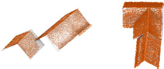
Figure 8: Fitting results obtained on adjacent roofs. Left : two gable roofs. Right : a gable T-shaped roof and a simple gable roof. When fitting onto a specific roof, the other one is considered as part of the outlier distribution.
