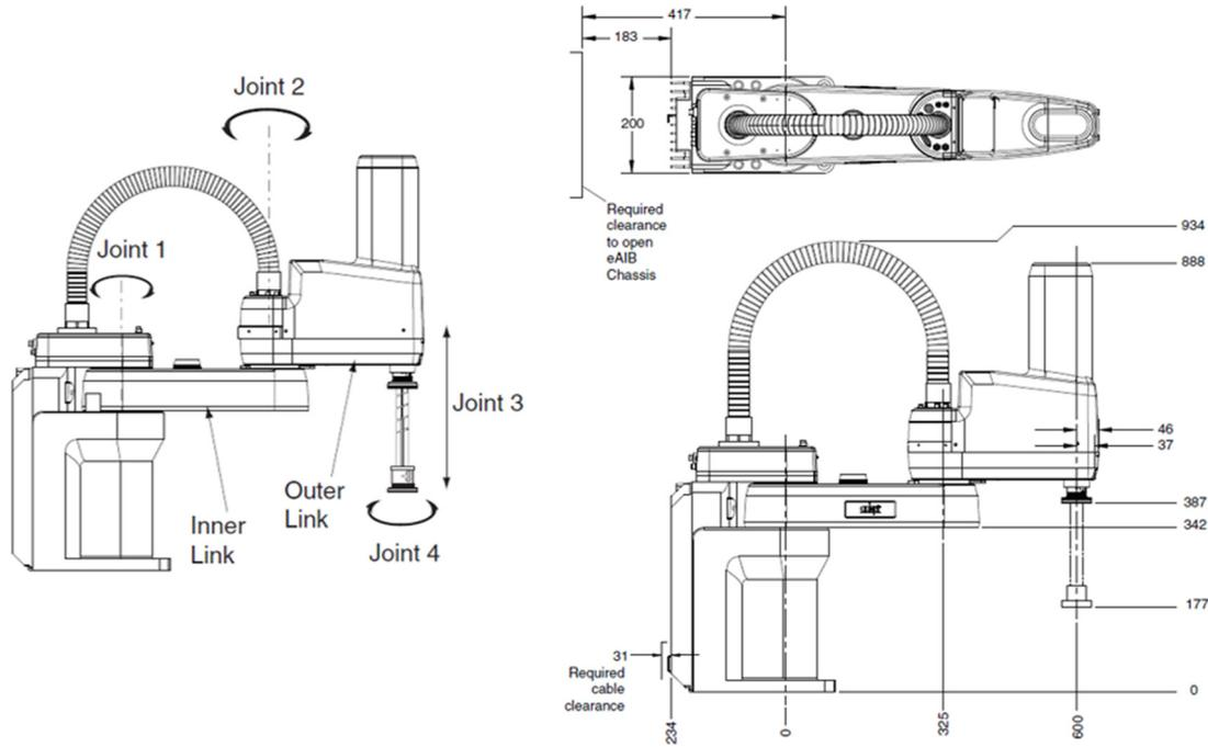
Fig. 3. Adept Scara Cobra S600 robot dimensions.
