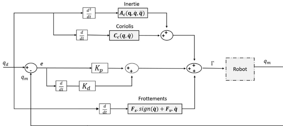
Fig. 14. Feedforward control.
