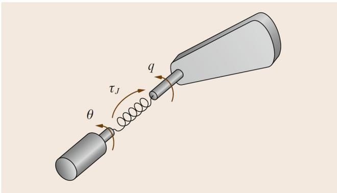
Fig. 2. Schematic representation of a flexible joint robot [7].
