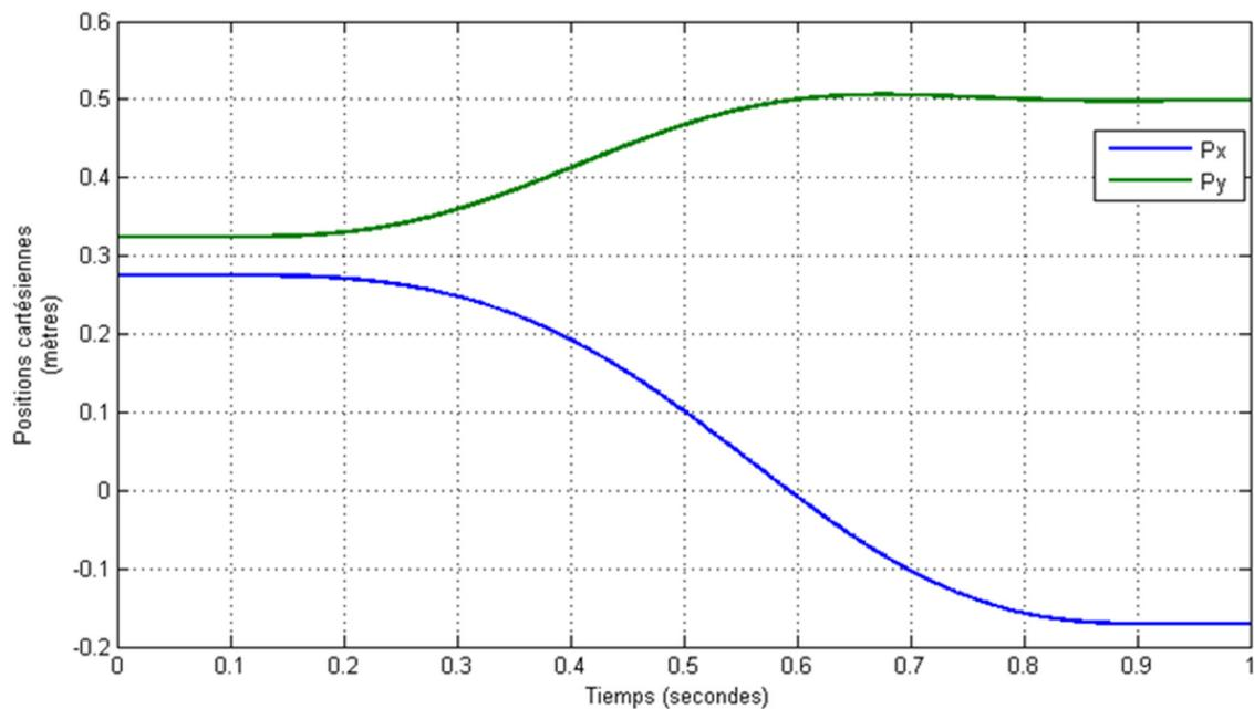
Fig. 11. Program tool path in the cartesian space.
