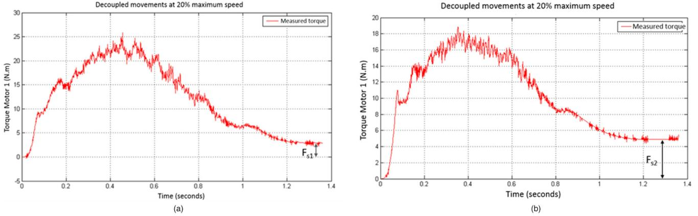
**Fig. 8.** Dry friction identification. (a) Dry friction joint 1. (b) Dry friction joint 2.
