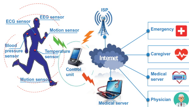
Figure 1: Framework for intelligent health care monitoring systems (HCMS) [5].
