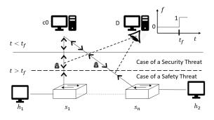
Fig. 1. Architecture proposed (c0: nominal controller, D: the detector,  $h_1$  and  $h_2$ : two hosts,  $s_1$  and  $s_n$ : the switches and  $t_f$ : the time of the failure or the beginning of the attack)
