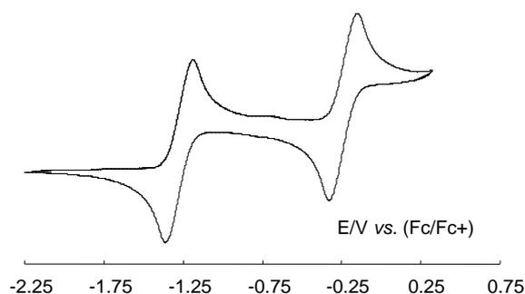
**Figure 2.** Cyclic voltammogram of a THF solution of compound  $\text{MoCl}_2(\text{iPr}_2\text{dad})_2$ .
