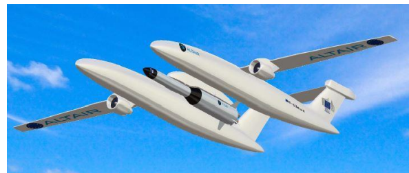
Fig. 8 View of the carrier with the launcher attached
