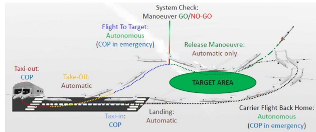
Fig. 7 ALTAIR CONOPS: COP (Carrier Operator) vs. Autonomous Operation
