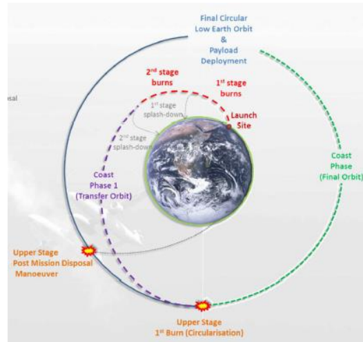
Fig. 14. Orbital module mission profile
