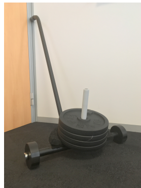
Figure 4: Two wheeled trolley used for rolling noise tests: shown here with 20 kg added mass.
