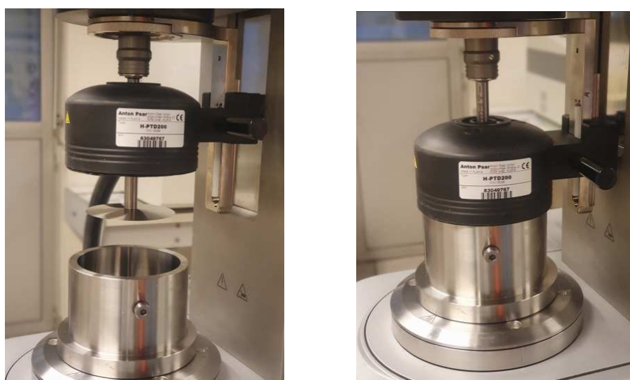
Figure 5. The newly designed interfacial rheology setup, shown in open position (left) and in closed position (right).
