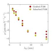
Fig. 7 Electrophoretic mobilities of grafted and adsorbed F108 brushes. Grafted and adsorbed F108 brushes show similar variations of the electrophoretic mobility of particles  $\mu$  with the Debye length  $\lambda_{\rm D}$ . Red markers: TPM particles with F108 grafted on the surface before polymerization. Yellow markers: TPM particles with saturated adsorbed F108, washed by several cycles of centrifugation and resuspension in de-ionized water.
