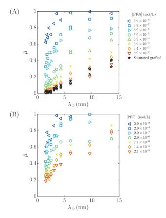
Fig. 5 Polymer adsorption probed by Debye length sweeps. (A) Reduction of the normalized mobility with  $\lambda_D$  for TPM colloidal particles with adsorbed F108. (B) Reduction of the normalized mobility with  $\lambda_D$  for the same TPM colloidal particles with adsorbed PEO.
