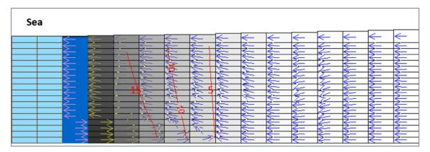
**Figure 11.** Simulated state of equilibrium of the seawater intrusion in the area of Ambabbo. NS vertical cross-section. Concentration in kg/m<sup>3</sup>.
