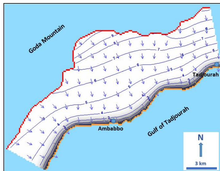
Figure 10. Simulated piezometry corresponding to the equilibrium state of the seawater intrusion.
