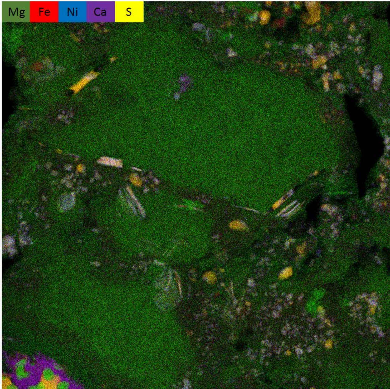
1528 1529 Fig. S5. An Mg-Fe-Ni-Ca-S x-ray map of the area of the matrix of NWA 12563 in Fig. 16, showing 1530 phyllosilicate-rich patches (green) and porous multi-phase regions with amorphous silicate and sulfide 1531 inclusions. Width of image \sim 9 \mu\text{m} .
