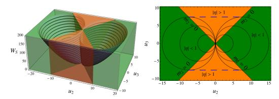
Figure 2. Sadowsky's energy surface  $W_S(u_2, u_3)$  from equation (8). The energy surface is made up of two symmetric wells. Level sets are shown in black, and the 'forbidden' region corresponding to  $|\eta| = |u_3/u_2| > 1$  is shaded in orange (see section 4). Left: three-dimensional plot. Right: contour plot, with a level set of the convexified functional from Freddi et al. [2015] shown in dashed blue.
