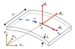
Figure 1. A ribbon with width w, thickness h is seen as a one-dimensional elastic structure with centerline r(s) and Cosserat local frame  $\{d_1(s), d_2(s), d_3(s)\}$ , parametrized with the arclength s.
