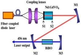
Fig. 2. Schematic diagram of experimental settings for the doubled frequency of the 456 nm blue laser; the distance from S1 to M1, from M1 to M2 and from M2 to M3 mirrors are 110, 400 and 56 mm, respectively [27].
