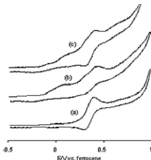
**Figure 11.** Effect of the addition of  $[\text{Bu}^n_4\text{N}][\text{Cl}]$  and  $[\text{Bu}^n_4\text{N}][\text{Br}]$  on the cyclic voltammogram of  $\text{MoI}_3(\text{PMe}_3)_3$  in  $\text{CH}_2\text{Cl}_2$ . (a) Without added salts; (b) with added  $\text{Cl}^-$ ; (c) with added  $\text{Br}^-$ .
