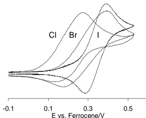
**Figure 4.** Cyclic voltammetry of complexes  $\text{MoX}_3(\text{PMe}_3)_3$  ( $\text{X} = \text{Cl}, \text{Br}, \text{I}$ ) in  $\text{CH}_2\text{Cl}_2$ . Supporting electrolyte =  $\text{Bu}_4\text{NPF}_6$ .
