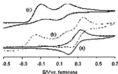
**Figure 7.** Effect of the addition of [Pr<sup>n</sup><sub>4</sub>N][I] on the cyclic voltammogram of MoI<sub>3</sub>(PMe<sub>3</sub>)<sub>3</sub> in CH<sub>2</sub>Cl<sub>2</sub>. (a) Without I<sup>-</sup>; (b) with added I<sup>-</sup>; (c) voltammogram of [Pr<sup>n</sup><sub>4</sub>N][I].
