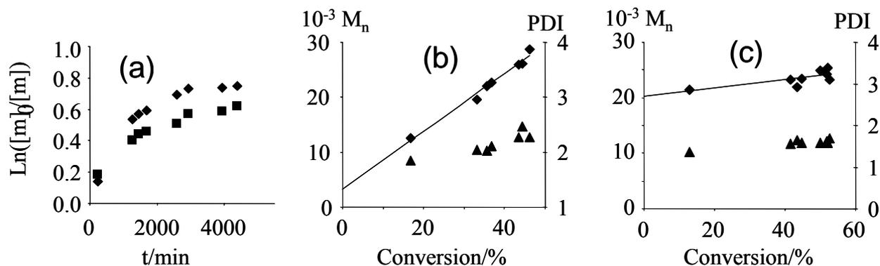
**Figure 2.** Styrene polymerization in toluene (30% v/v) at 80°C in the presence of  $\text{MoX}_3(\text{PMe}_3)_3$  and AIBN. Styrene/ $\text{Mo}^{\text{III}}$ /AIBN = 200/1/0.64 ( $X = \text{Cl}$ ); 250/1/0.64 ( $X = \text{I}$ ): (a) 1<sup>st</sup> order kinetics (squares: Cl; diamonds: I); (b)-(c):  $\overline{M}_n$  (diamonds) and PDI (triangles) as a function of conversion for  $X = \text{Cl}$  (b), I (c).
