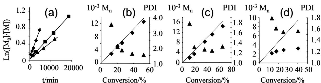
**Figure 1.** Styrene polymerization in toluene (30% v/v) at 90°C in the presence of  $\text{MoX}_3(\text{PMe}_3)_3/\text{BEB}$  (X = Cl, Br, I): (a) 1<sup>st</sup> order kinetics (diamonds: Cl; squares: Br; triangles: I); (b)-(d):  $\overline{M}_n$  (diamonds) and PDI (triangles) as a function of conversion for X = Cl (b), Br (c) and I (d). The straight lines correspond to the theoretical  $\overline{M}_n$  values. Styrene/ $\text{Mo}^{\text{III}}$ /BEB = 251/1/1 (b); 244/1/1 (c); 225/1/1 (d).
