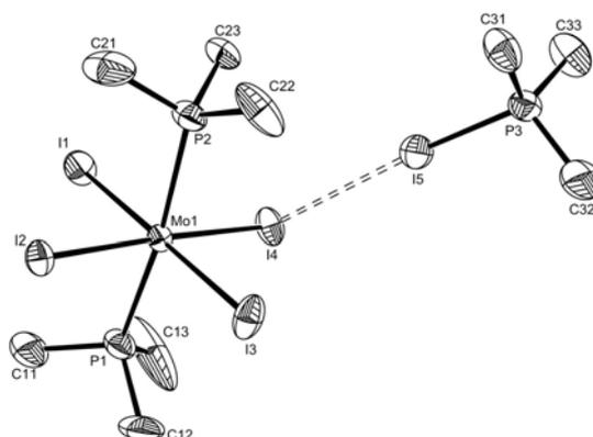
**Figure 13.** An ORTEP view of the  $[\text{PMe}_3][\text{MoI}_4(\text{PMe}_3)_2]$  molecule.
