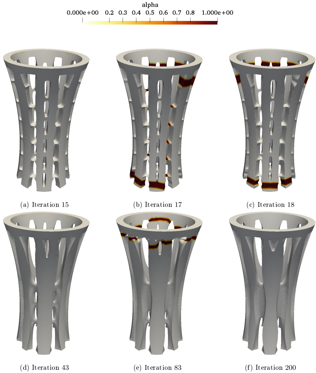
Figure 31: Damage variable \alpha at the final time T plotted for several optimization iterations for the shape in Fig. 30c
