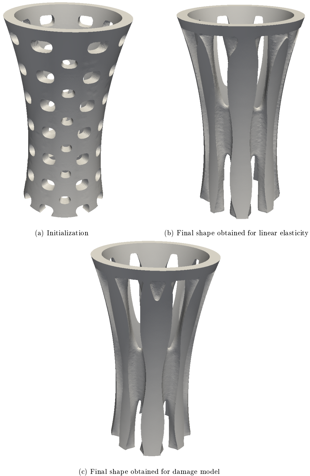
Figure 30: Column shapes for a fine mesh and the imposed displacement (61)
