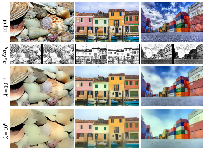
Fig. 10. Edge-preserving decomposition. Our method can also generate edge-preserving multiscale decompositions of an image, which can be further used for applications such as tone mapping, detail exaggeration, etc. All these images presented here have a size of 1280 \times 800 , and use gradient-based diffusion coefficient a_x and a_y , for two different diffusion times \lambda .
