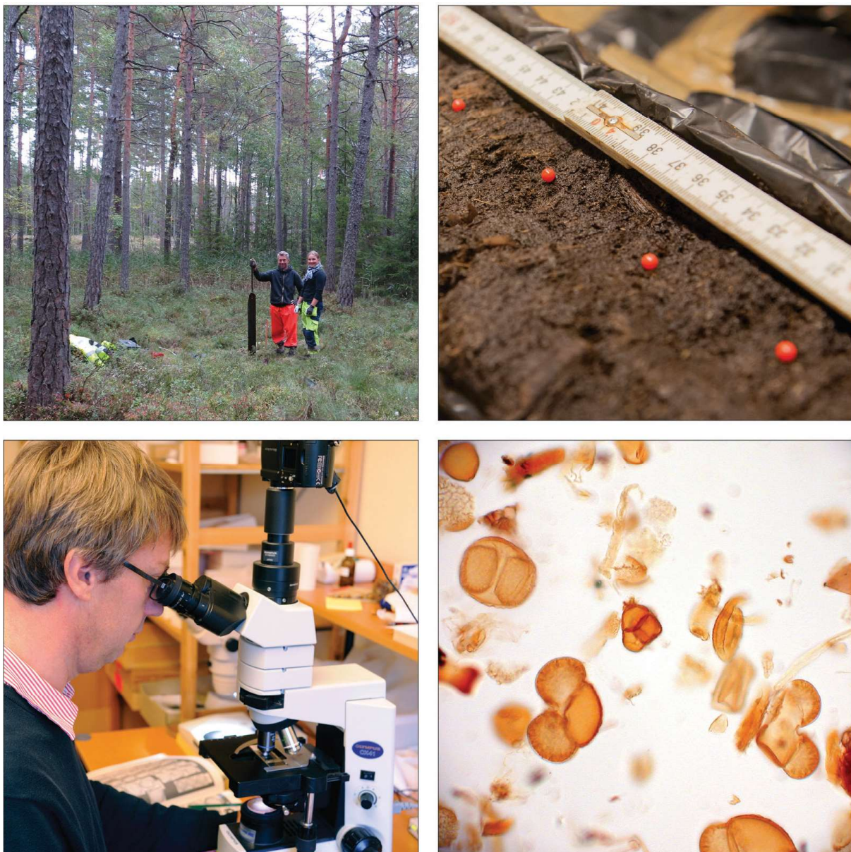
Fig. 4. The basic steps of pollen analysis, from peat coring on a bog, via subsampling to microscoping. The pollen photo is taken at magnification \times 400 (photos: Per Lagerås and Henrik Pihl)
