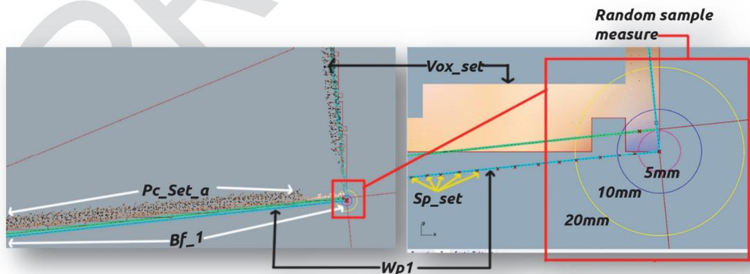
Figure 7. Accuracy test- **LEFT**, sample segment on a PC\_Set slice. **RIGHT**. Reference distances around a random sample point for measuring. Measured points are contained within a voxel set from which wall paths are retrieved
