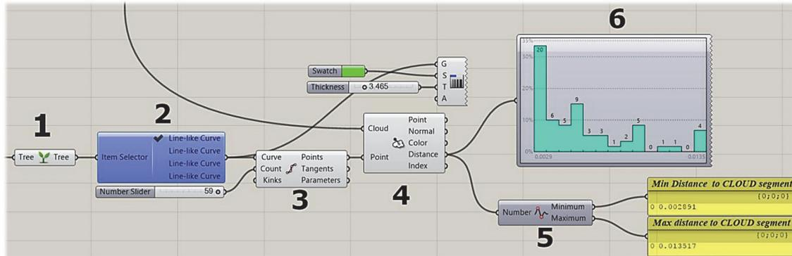
Figure 8. Accuracy measurement tool. **1** Wall footprint set (as tree); **2** Wall footprint selector; **3** sample point creator; **4** PC\_Set closest point component; **5 and 6** Measurements.
