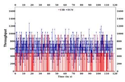
Fig. 8: Troughput comparison: sending interval of control messages = exponential 15ms.
