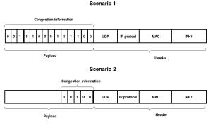
Fig. 3: Example of packets with CIB.
