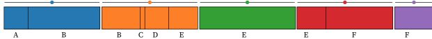
Figure 2: The cumulative binning process splits multiple categories (A, B, C) which are cumulative values (e. g., by days) into regular bins (represented as top horizontal lines). As a result, bins contain the same number of values (except probably the last one which is not filled, yet), but that may be from multiple categories/days (e. g., blue A, B) or the same day (e. g., green E).
