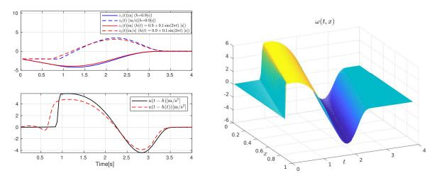
Fig. 2. On the left: evolution of the states of the double integrator with input delay  $(h=0.9[\mathrm{s}])$  (blue lines), and slowly time-varying delay  $(h(t)=0.9+0.1\sin(2\pi t)[\mathrm{s}])$  (red lines) when stabilizing with the prescribed-time predictor control (60) (black line). On the right: numerical solution of the transport PDE  $\omega(t,x)$  in (29).
