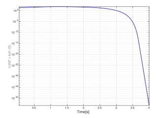
Fig. 3. Evolution of  $\|z(t)\|^2 + \|\omega(t,\cdot)\|_{L^2}^2$  (plotted in logarithmic scale) of the closed-loop system with the prescribed-time predictor control (60) where  $h=0.9[\mathrm{s}]$  and  $T=3\mathrm{s}$ .
