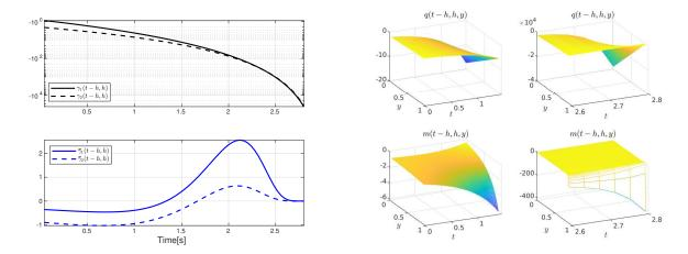
Fig. 1. On the left: evolution of the time-varying gains  $\gamma$  (plotted in logaritmic scale) in (38) and  $\bar{\gamma}$  in (46) at x=h. On the right: evolution of the time-varying kernel gains q in (37) and m in (45) at x=h, on two different time intervals.
