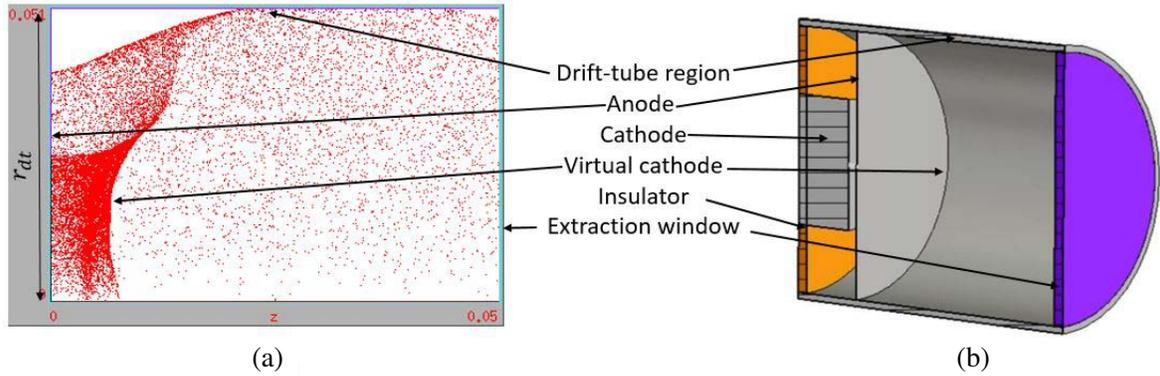
**Figure 19.** Vircator model simulated using (a) XOOPIIC and (b) CST-PS.
