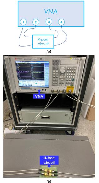
FIGURE 6. Configuration of the resistorless H-tree prototype experimental setup.
