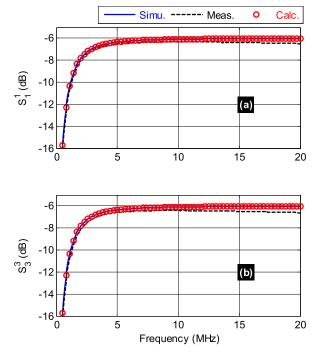
**FIGURE 7.** Comparisons between simulated, measured and calculated reflection coefficients of the H-tree circuit prototype: (a)  $S_1^1 = S_2^2$  and (b)  $S_3^3 = S_4^4$ .
