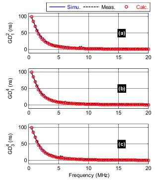
**FIGURE 10.** Comparisons between simulated, measured and calculated GDs from transmission coefficients, (a)  $S_1^2$ , (a)  $S_1^4$  and (a)  $S_3^4$  of the H-tree circuit prototype.
