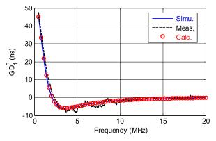
**FIGURE 11.** Comparisons between simulated, measured and calculated GDs from transmission coefficient,  $S_1^3$  of the H-tree circuit prototype.
