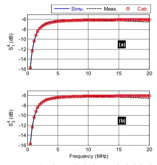
**FIGURE 9.** Comparisons between simulated, measured and calculated transmission coefficients of the H-tree circuit prototype: (a)  $S_1^4 = S_2^3$  and (b)  $S_4^3 = S_4^3$ .
