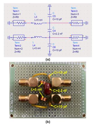
FIGURE 5. (a) Schematic and (b) photograph of the resistorless H-tree prototype.
