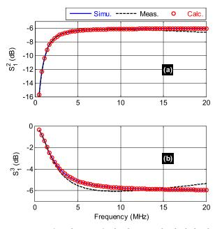
**FIGURE 8.** Comparisons between simulated, measured and calculated transmission coefficients of the H-tree circuit prototype: (a)  $S_{21} = S_{43}$  and (b)  $S_{31} = S_{42}$ .
