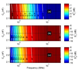
**FIGURE 17.** Mappings of (a)  $S_1^3$ , (b)  $S_1^1$  and (c)  $S_3^3$  magnitudes versus  $(f, C_0)$ .
