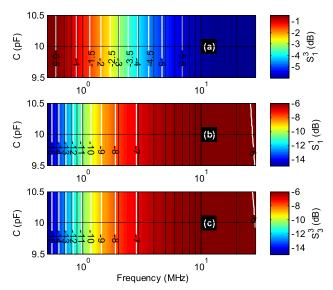
**FIGURE 15.** Mappings of (a)  $S_1^3$ , (b)  $S_1^1$  and (c)  $S_3^3$  magnitudes versus (f, C).
