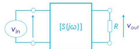
FIGURE 8. Illustrative diagram to generate the time-domain response of system S(j\omega) .
