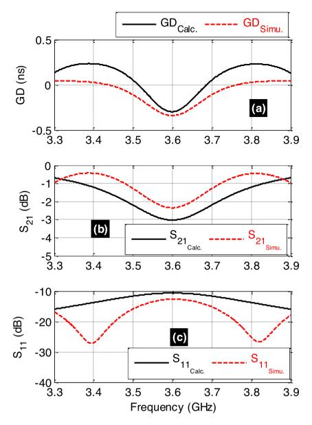
**Figure 8.** Calculated and simulated (a) GD, (b)  $S_{21}$  and (c)  $S_{11}$  of BP NGD circuit shown in Figure 5.
