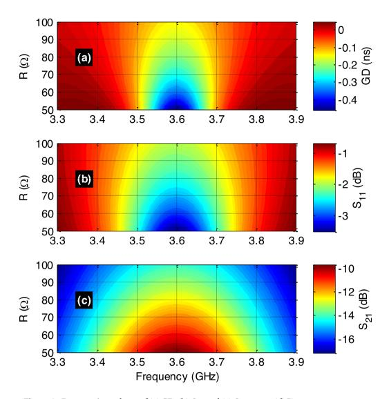
**Figure 6.** Parametric analyses of (a) GD, (b)  $S_{21}$  and (c)  $S_{11}$  versus (f, R).
