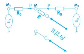
Figure 4. Open-ended stub based NGD passive circuit.
