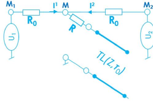
**Figure 4.** Open-ended stub based NGD passive circuit.
