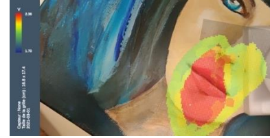
Figure 2 : Screenshot of the mobile application with a superimposition of the camera view and the THz image.
