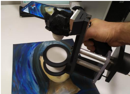
Figure 1 : Photography of the experiment. A painting is manually scanned using the AR-THz system.
